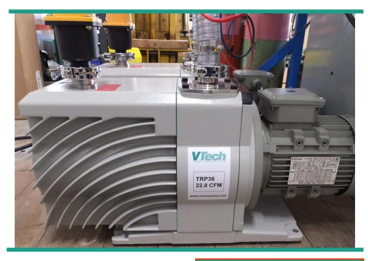
The **VTech TRP Series High Vacuum Pumps** have been designed to meet the needs of industrial users for non-corrosive environment applications such as Air Conditioning and Refrigeration manufacturing. They are utilized for both pre-evacuation carousels as well as integrated into VTech leak testing and refrigerant charging equipment.
